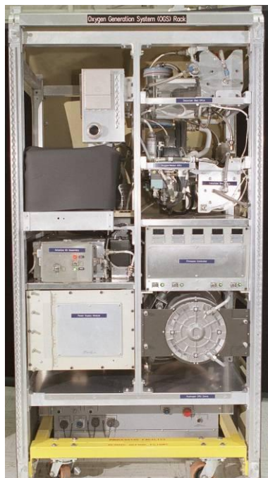
Figure 2: A mock-up of the Oxygen Generation System (OGS) located in the Tranquility Module on the ISS
